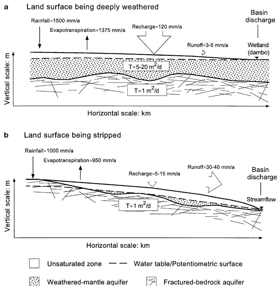
fractured bedrock and, in places, by localised aquifers in the weathered mantle. Discharge is in the form of highly variable streamflow that results from the high runoff component and the fact that the thinner weathered mantle reduces buffering of the basin inputs (runoff, recharge).
