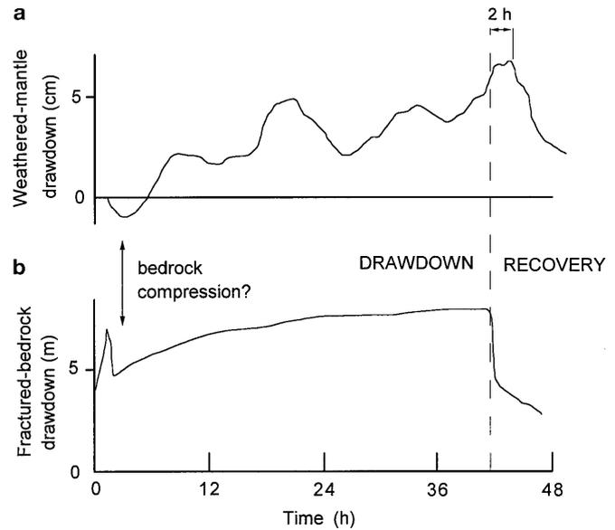
**Figure 12** Relation between drawdown and time (linear plot) in **a** weathered mantle and **b** fractured bedrock, for a 2-day pumping test at borehole CD0360 in the Nyabisheki catchment
