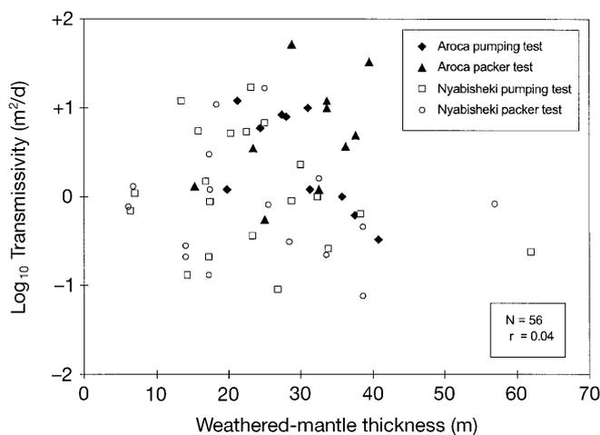
**Figure 11** Relation between (1) log<sub>10</sub> bulk transmissivity of the fractured-bedrock aquifer, determined by packer testing and pumping tests in both study areas, and (2) thickness of weathered mantle, indicated by depth of borehole casing
