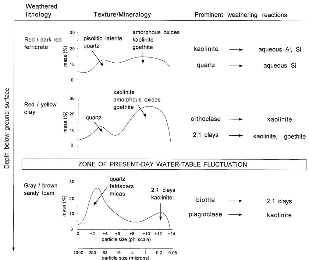
**Table 1** Textural analysis of weathered-mantle aquifer, Aroca catchment. *mbgs* Metres below ground surface
