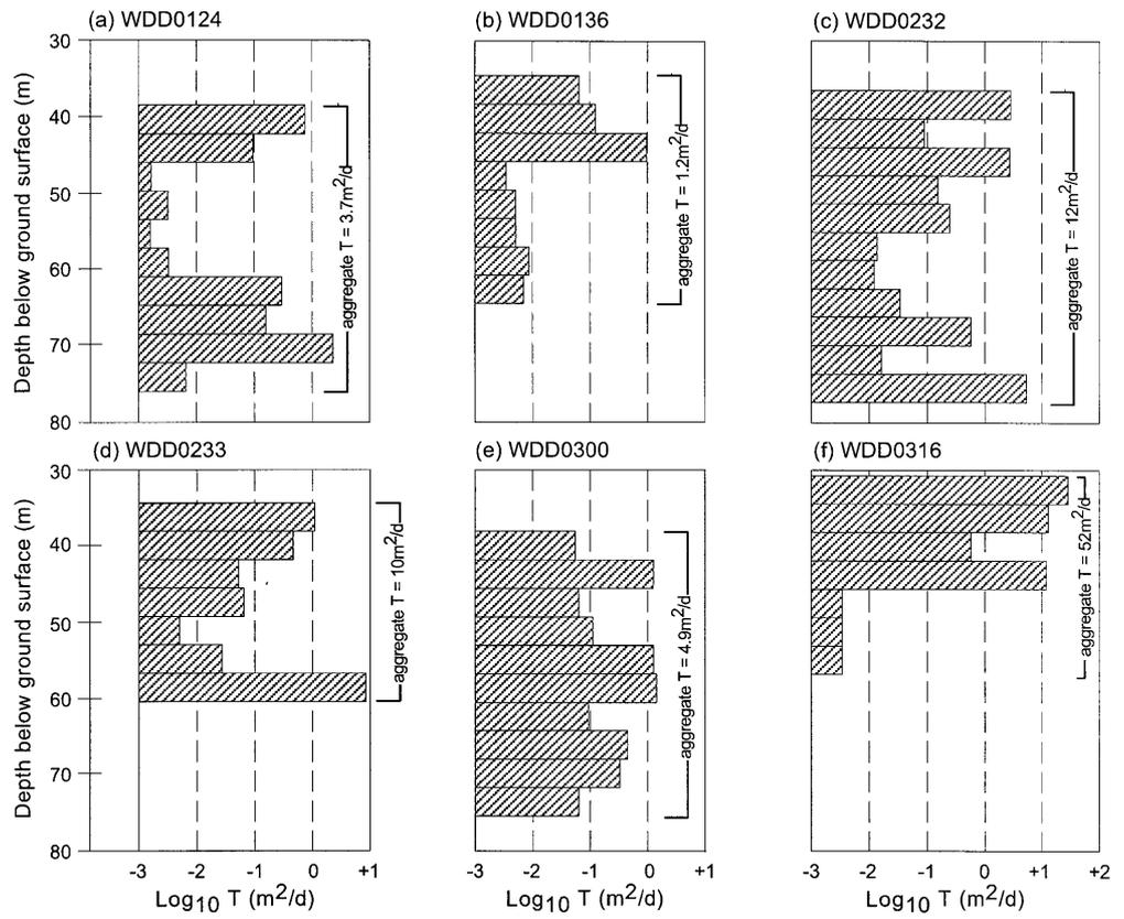
**Figure 7** Relation between  $\log_{10}$  transmissivity ( $T$ ) of tested fracture zones and depth for five sites in the Aroca catchment:
