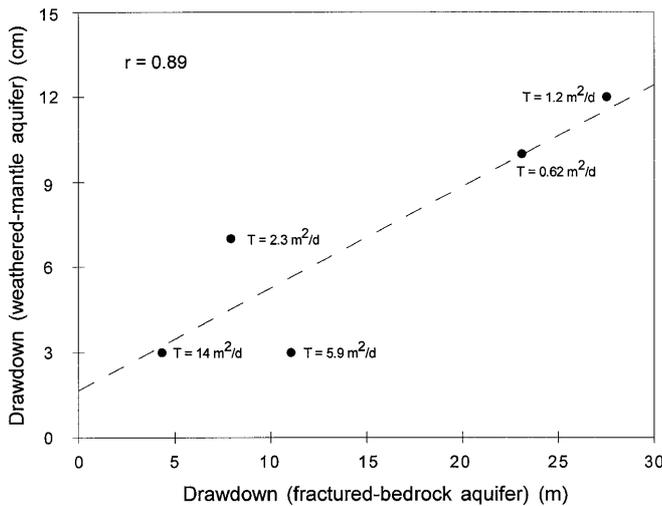
**Figure 13** Relation between drawdown in weathered mantle and drawdown in fractured bedrock during pumping tests of 1–2 days' duration at five sites in both study areas
