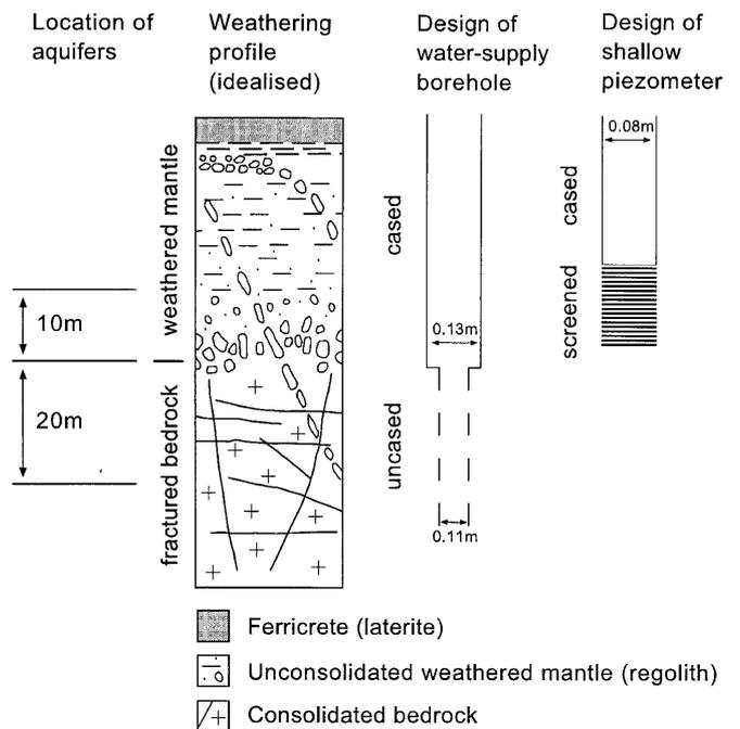
**Figure 2** Vertical representation of the weathered crystalline-aquifer system, including locations of aquifers and construction of wells
