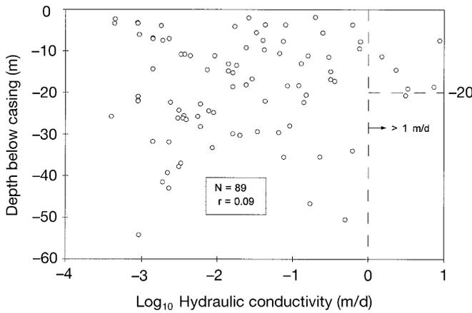
**Figure 8** Relation between depth below well casing (i.e., below bedrock surface) and  $\log_{10}$  of hydraulic conductivity for packer-tested zones in the fractured-bedrock aquifer of the Aroca catchment
